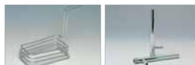
Cooling coil Aspirators
