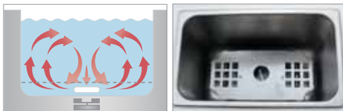
Powerful circulation by built in agitator
