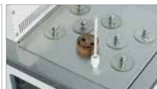
Easy holding of U-shaped viscometer glass tubes (optional)
