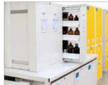
Superiorly chemical resistant PP trays included with the drawers keep lab material safely tidy and organized.
