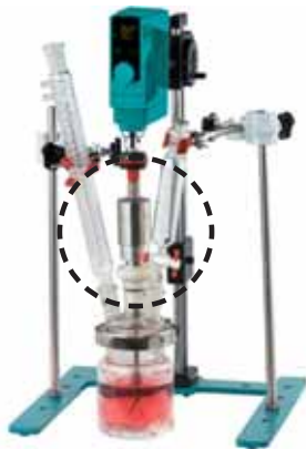
Application of magnetic drive
